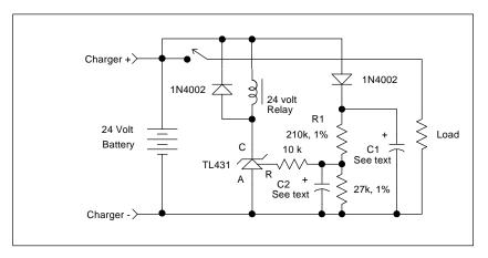
In this circuit, the battery will buffer the load from the charger a bit but the load will not receive power until the battery voltage has risen above the set-point.
